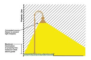
Light Fixture Orientation and Shielding
